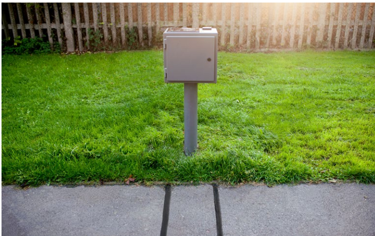
RidePod® BP in the MetroCount cabinet, installed on a shared path to record bikes and people.
