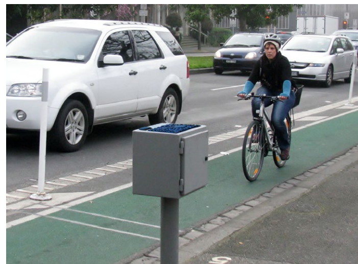
VicRoads record bikes at around 40 sites both on and off road with the RidePod® BP.
