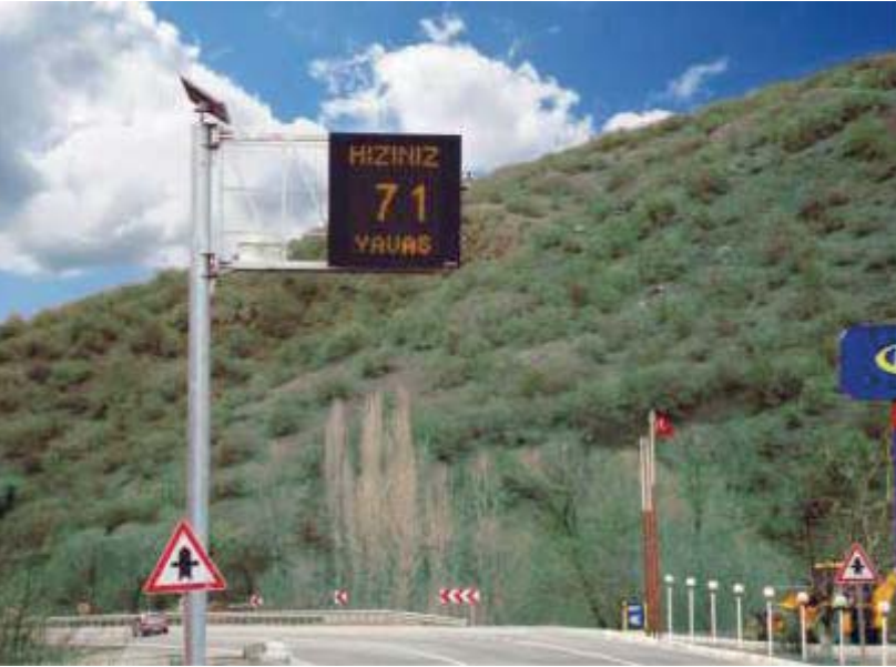
RADOR 101, Doppler Radar Speed Warning Sign, SAMSUN / 2010 RADOR 101, Doppler Radar Hız İkaz Sistemi, SAMSUN
