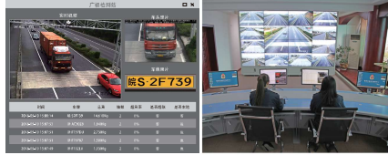
The platform shows vehicle picture and corresponding vehicle information such as plate number and gross weight
