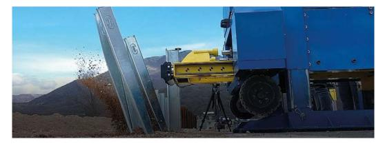
The instrumentation is remotely controlled by radio: the movement of the vehicle, the positioning of the hammer impacting the post, the height of the impact, and the impact energy may be easily set up.
