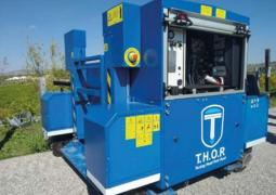
The four steering wheels move longitudinally and transversely, allowing a rapid and appropriate positioning for the test. Thanks to its small dimensions, T.H.O.R 3 may work on the emergency lane.
