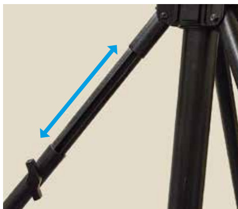
Extendable tripod leg for uneven slopes
