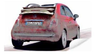
Car plate reading cameras may face a situation in which dirty plates quickly alternate with clean and bright plates. It is very important in this case to use pulsed and adaptive floodlights which adjusts to
