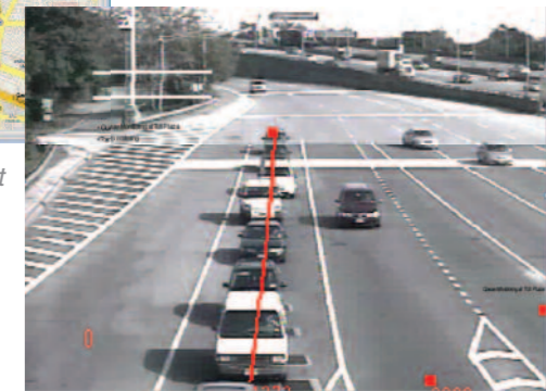
Queue Monitoring at Toll Plazas
