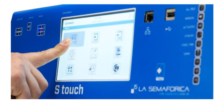
La Semaforica's Cartesio Traffic Controller met the latest transportation industry standard, which incorporates the Linux open architecture operating system.
