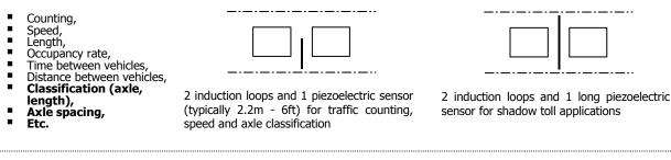
HERA W : Weigh-in-Motion, automatic classification and traffic counting based on axle spacing, length, etc.
