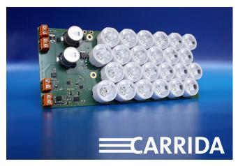
by activating several connected VC Flash modules. The module measures 195 x 80 x 20 mm. It operates with a central wavelength of 850 nm and a spectral width of 30 nm. Power consumption peaks at 36 W for the highest pulse duration and pulse frequency levels. ...
