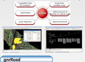
The most important characteristics of gnrRoad Simultaneously check out horizontal, longitudinal alignment, construction cost, mass curve to consequence of geometry modification.
