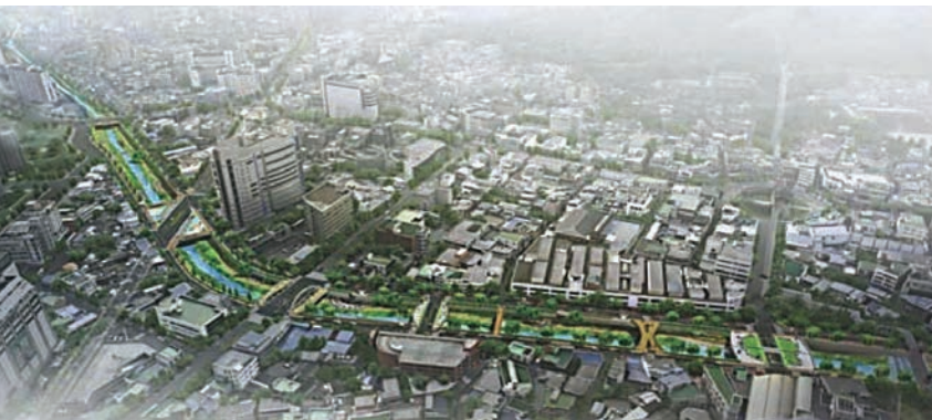
Suwon Stream Renaissance Project, Suwon City, Korea: Demolition of concrete covered CBD section to restore the eco-system and create riverside public amenity spaces, six new road bridges and two pedestrian foot-bridges.
