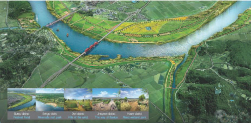
The Geum River Improvement Project – Section 5 (Buyeo District), Korea: Improvement of river regime for climate change adaptation and preservation of river ecology; Restoration/Improvement : 9.08km / Riverbank Reinforcement: 6.07km ; River channel dredging of 5,370,000 \text{ m}^3 ; Flood control and drainage structures at 9 places ; Bicycle lane 22.4km and creation of ecology park, cultural and leisure activity spaces
