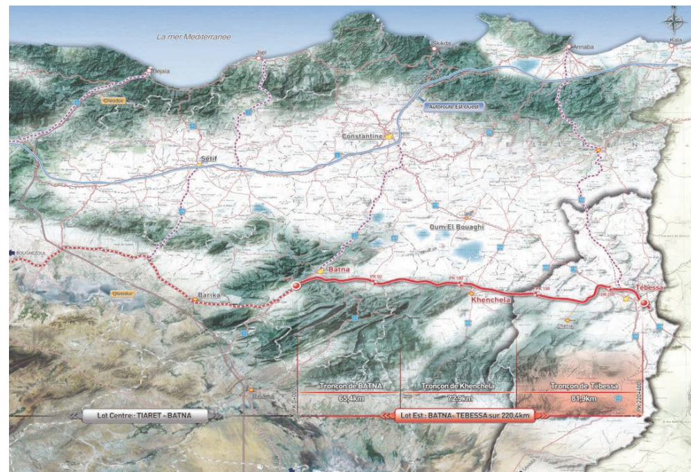
High Plateau Bypass Expressway (Rocade des Hauts Plateaux), Algeria: Basic & Detailed Design of 4 to 6 lane Expressway, 220.4km w/ 17 Interchanges, 105 Bridges & 9 Rest Areas
