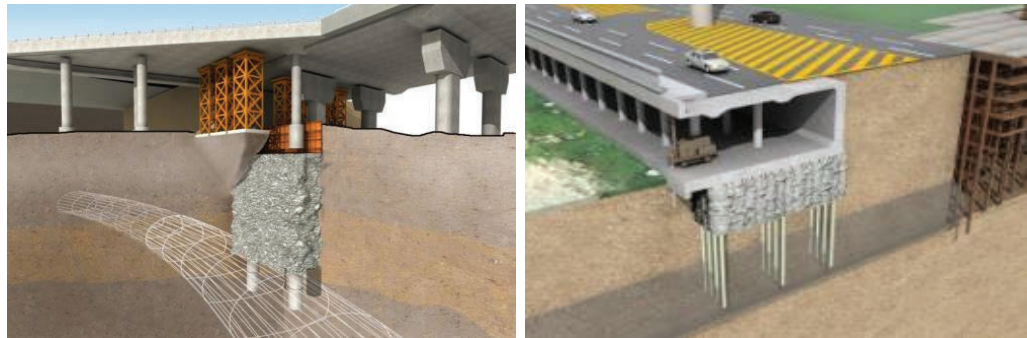
Construction of Busan Light Rail Transit, Korea: Strengthening of Foundations for the Existing Structures of LRT tunnel and Piling Works
