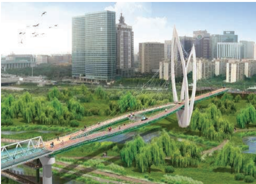
Yoido Eco-Stream Park Pedestrian Bridge, Korea: Composite Cable-stayed Bridge with V-shaped Inclined Pylon
