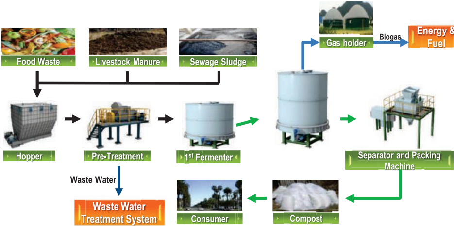
An Organic Waste to Energy Plant Process
