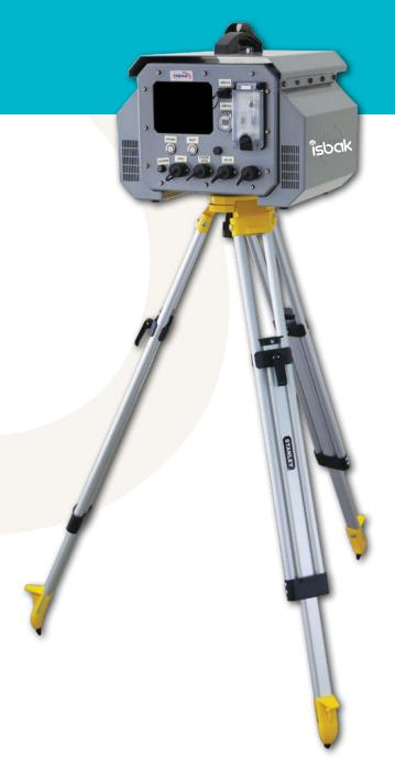
developed by ISBAK, there will be less operator dependency. It obtains all the parameters related to the road, where the radar is installed, in few seconds with the help of the artificial intelligence technology. With this technology, operator-based false parameter entries can be prevented.
