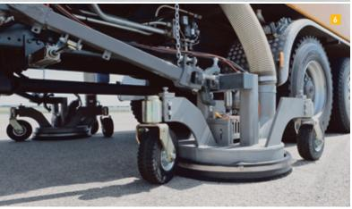
Every surface is faced under heavy traffic load to change the structure of the surface texture gradually. If the measured friction values fall below a certain level described in international or national regulation, it must be restored by either cleaning or retexturing the surface structure.
