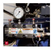
system can only be activated when the vehicle is actually in motion. Even at the full load (2,750 bar and 29 l/min, at a vehicle speed of 4.8 km/h) the water and debris is entirely withdrawn by suction into the waste water tank.
