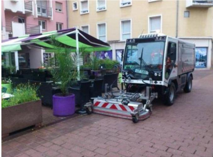
The **OSC 5000** is built on a LADOG chassis 1250 (German production) and is ideal for cleaning larger surfaces and oil spills and other kind of contamination – e.g. chewing gum.
