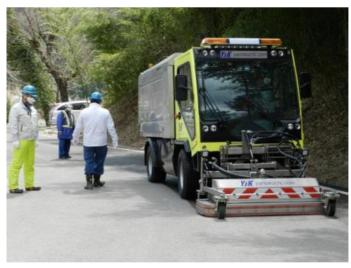
The **OSC 7000** is built on a LADOG chassis T 1550 (German production) and is ideal for cleaning larger surfaces and oil spots and tracks and for special cleaning of sports surfaces, construction site cleaning and gum removal on traffic areas.
