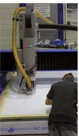
Numerical plastic and steel plate processing unit
