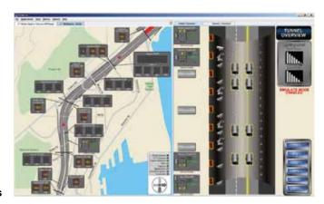
The user interface is customized for each project to minimize the number of steps required to respond to emergencies. This application allows operators to implement a complete response to an event such as a tunnel fire in as few as five mouse clicks in less than 20 seconds.
