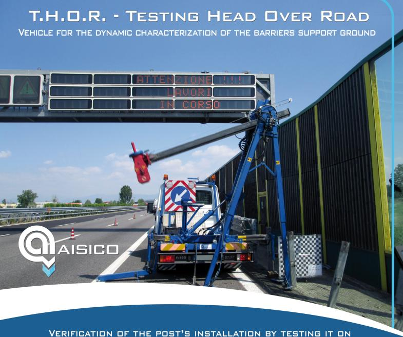
VERIFICATION OF THE POST'S INSTALLATION BY TESTING IT ON THE ROAD AND COMPARING THE RESULTS WITH THOSE ONES PREVIOUSLY OBTAINED FROM THE SAME DEVICE DRIVEN INTO THE SOIL OF TEST HOUSE.
