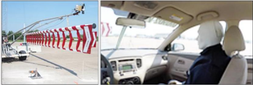
Versilis Horizontal Warning Gate (HSG-40CW) MASH Crash Testing at Texas A&M Transportation Institute's Certified Laboratory.
