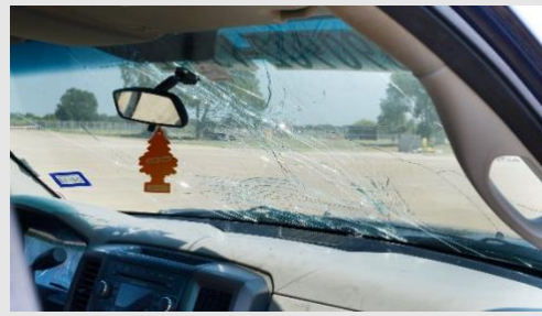
Minimal quantity of glass fragments into occupant compartment
