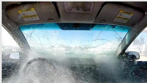
Important quantity of glass fragments into occupant compartment
