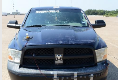
After crash - minor windshield damage
