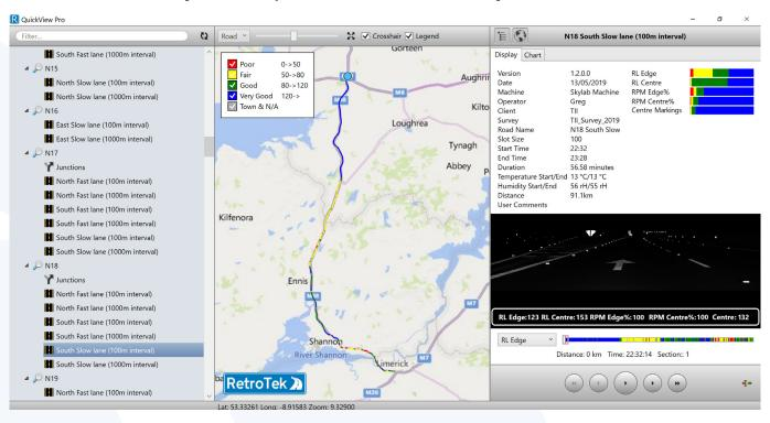
Measurements are processed in real-time and results are available immediately. The QuickView software provides instant reports at the end of each survey showing all results averaged in 100 meter / 100 yard and 1km / 1 mile segments with flexible colour coded performance thresholds in various GPS tagged output formats – csv, kml, shp, pdf and video files. Reports are available on a removable USB memory device.
