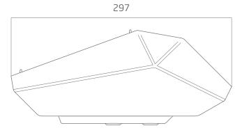
It can be mounted using universal brackets available in the market using two m8 inserts existing
